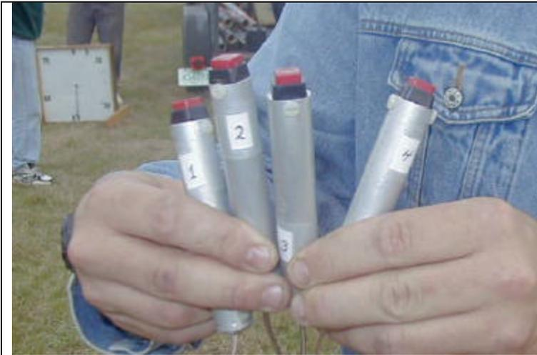
The switches that are used to flash the turn lights are “momentary on switches”; that is, you push and hold the switch to turn on the light. Purchase these switches at an electronic supply house. We used some  $\frac{3}{4}$  inch diameter aluminum tubing about 4 inches long with some machined end pieces to make a nice hand held housing.
