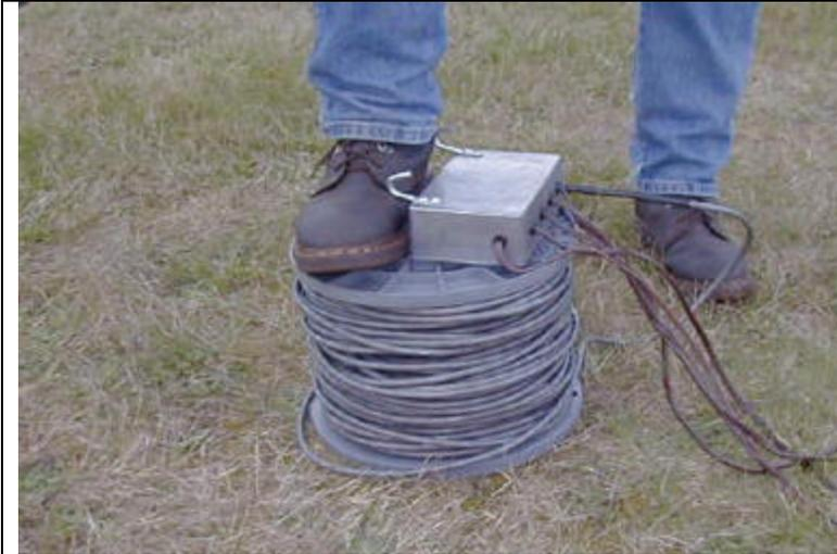
This system is light weight, simple & easy. The sheathed cable is less than  $\frac{1}{4}$  inch in diameter and the 350 feet of wire will roll onto a spool that is about 18 inches in diameter. Because the system is relay operated with the battery next to the relays, there are no line losses and the lights are bright. The 350-foot switch lines are just that, there is no time delay.
